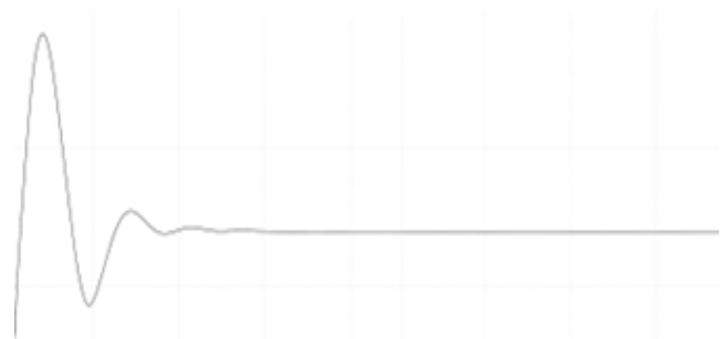
Figure 10: Simulation Result of AVR with PID Controller
