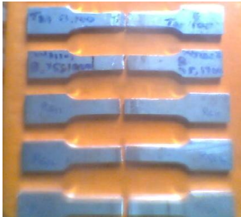
Figure .8 Tensile test specimens of Friction Stir Welded joints of AA7075 after.
