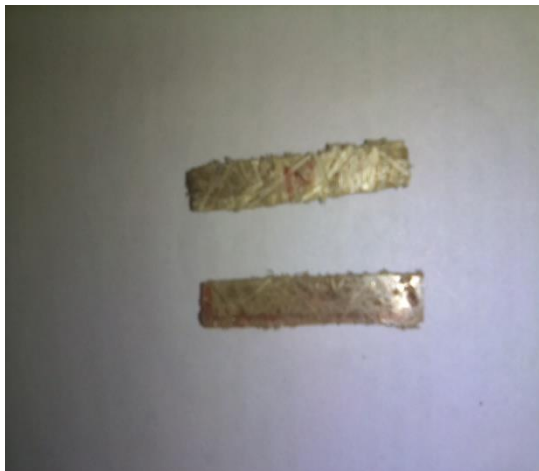
Fig.7 Tested specimen (Friction test)
