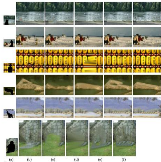
Fig. 4. (a) low-resolution pictures with missing areas in black; (b) Criminisi et al.'s results; (c) Patch Match results; (d) Diffusion-based results; (e) proposed methodology (the down sampling issue is ready to N = 4 ; patch size is 11 \times 11 ); (f) proposed methodology with N = 2 and patch's size of 15 \times 15 .
