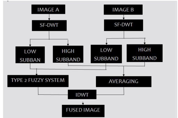
Fig. 1. Block Diagram Of Proposed Spatial Frequency DWT-Type2 Fuzzy Method
