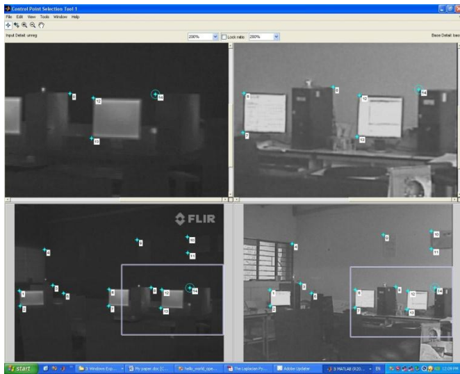
Figure 2. Usage of cpselect tool to mark reference points in the two images
