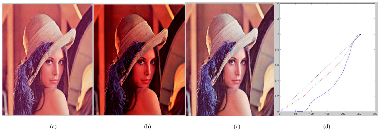
Figure 4. Results for image Lena . (a) Original Image, (b) Enhanced image obtained using HE, (c) Enhanced image obtained using the proposed algorithm, (d) Mappings for enhanced images : blue line indicates HE mapping, red dotted line indicates the proposed method and the dotted line indicates no change mapping.
