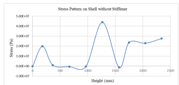
Fig. 6: Graph of Stress pattern on Shell without Stiffener
