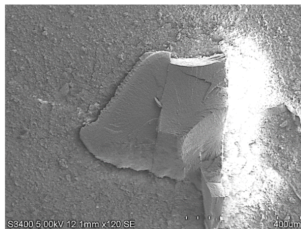
Fig. 4. SEM image of MP particle found to be of size ~0.5mm
