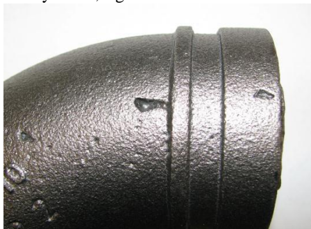
Figure 6 Blowhole of casting
