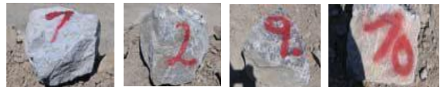
Figure 2. Four examples of the different rock block sizes dropped down along the Kloch slope profile. (Source: private documentation, 2011)
