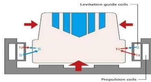
Fig 3: Stator and Rotor Coils Arrangement
