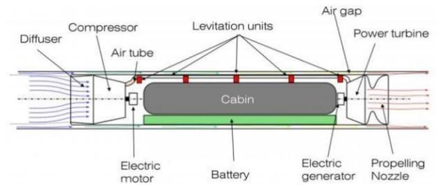
**Fig 9: Working of Hyperloop system**
