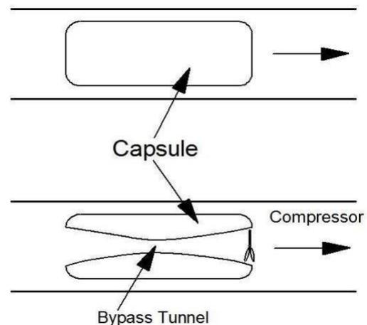
**Fig-10: Air through bypass tunnel**
