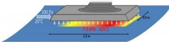
**Fig 7: Schematic of air bearing skis that support the capsule**
