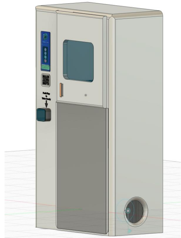
Fig. 1. HygieHelm prototype — CAD render of the floor-standing kiosk enclosure (400 mm \times 450 mm \times 900 mm). Left panel (front): LCD display, QR payment panel, and candy dispense chute. Centre: front-hinged door with viewing window and helmet cradle. Lower right: exhaust grille with polypropylene filter.
