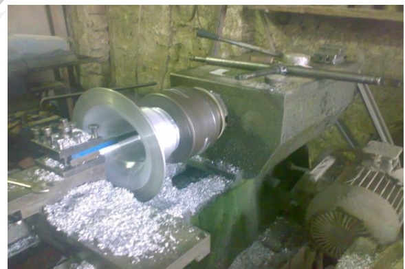
Figure (9).Bell-mouth fabrication through the study
