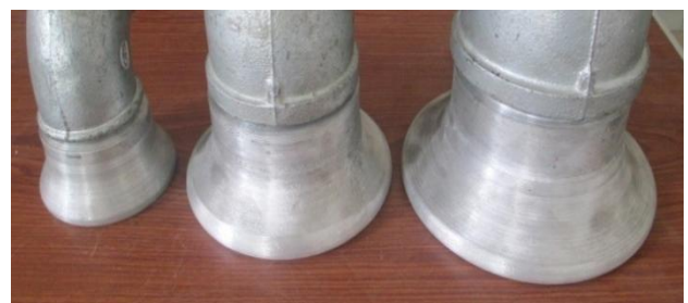
Figure (10).Three sizes of bell-mouth at same scale ratio with pipe diameter
