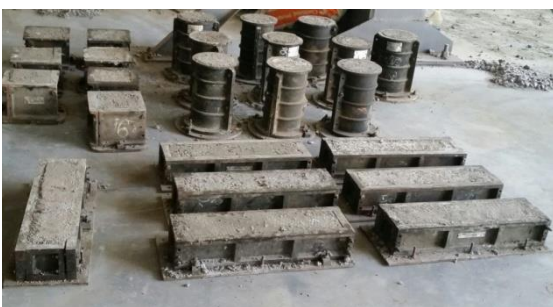
Fig.5 Casting of specimens
