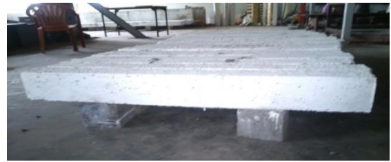
Fig.8 Beams after white washing
