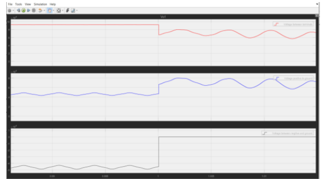
Fig. 7. Negative Pole to ground fault output Voltages
