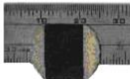
Figure 1 Photograph of PPy-PVAc composite film used as humidity sensor
