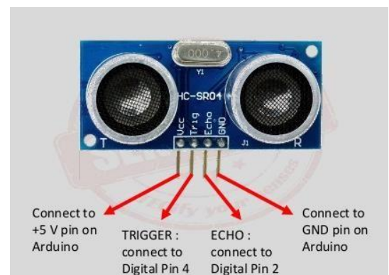
Fig.6: Ultrasonic Sensor HS-SR04. [4]
