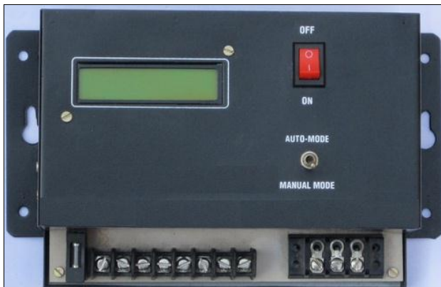
automatic tank water level controller with less I/Os for LCD and switches and button
