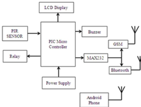
Fig1.Security System Block Diagram
