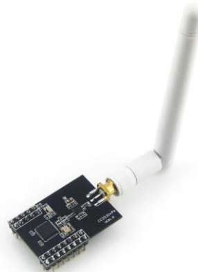
Figure 3: Zigbee Coordinator with Antenna
