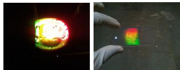
Fig .2: Symmetric pattern holograms after wet chemical processing
