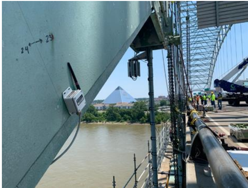
Figure 14 – Wireless sensors with strain gauge monitoring, accelerometers, and IoT devices that telemetrically communicate data.
