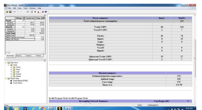
Fig.9. The Current (mA) and Power (mW) summary of the Proposed system
