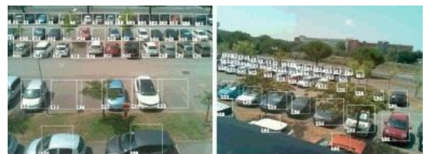
Fig 1: Occupancy detection using smart camera
