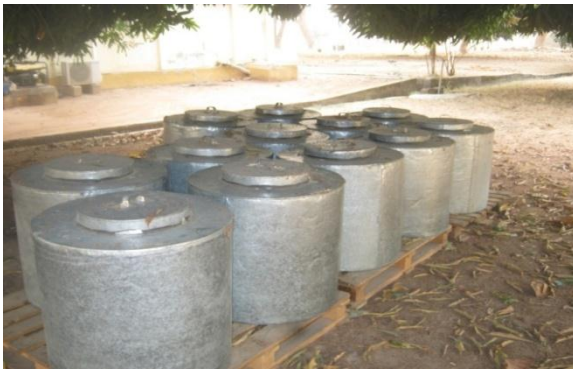
Plate .4. 300kg Aluminium hermetic containers set under a shade for storage.
