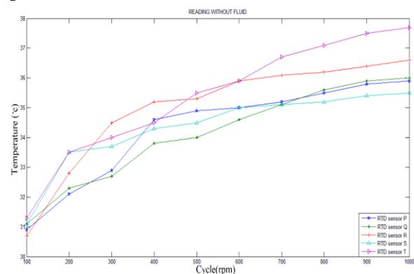
Graph 1: Arising temperature of shock absorber with air substance.
