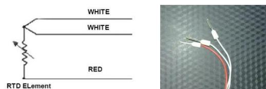
Figure 3 RTD sensors with line diagram
