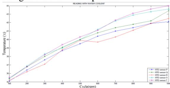
Graph 4: Graph temperature versus number of cycle for coolant substance
