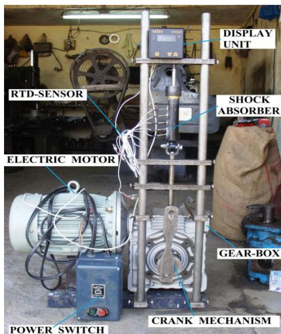
Figure 2 shock absorber test rig.
