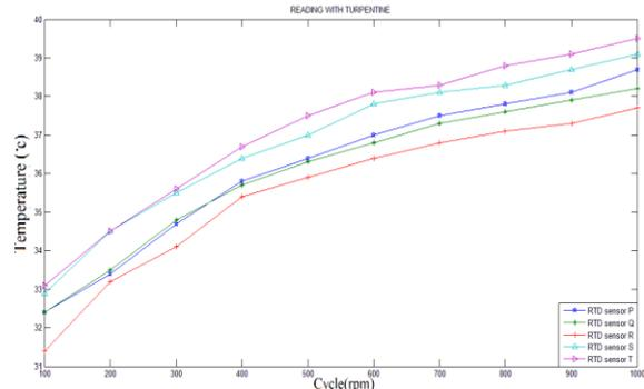
Graph 2: Graph temperature versus number of cycle with Turpentine substance
