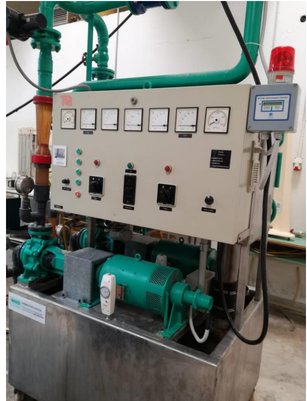
Fig. 1. Test facility for centrifugal pump testing
