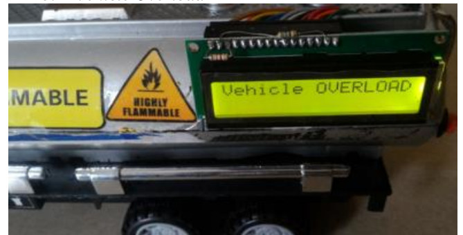
Fig 15. Vehicle Overload indication
