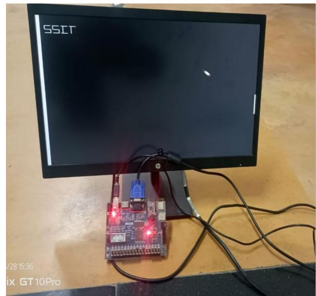
Figure 7: FPGA Pong Game Prototype with Real-Time VGA Output
