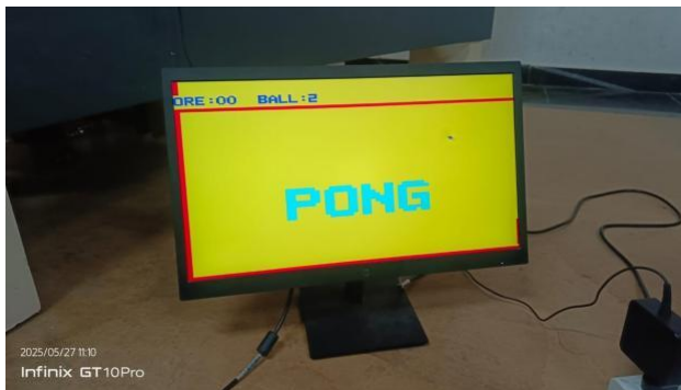
Figure 8: Real-time gameplay on VGA monitor showing the Pong interface with score and ball count display
