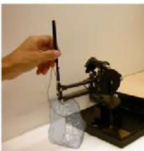
Figure 1: Haptic interfaces like the SensAble Phantom (pictured) allow a user to feel virtual objects through a pen-like tool.
