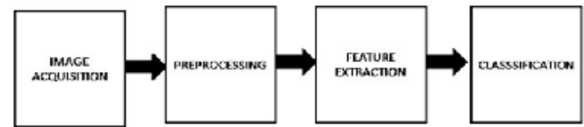
Fig : 2 Block Diagram of hand gesture recognition system
