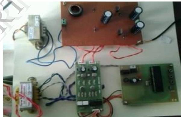
Fig.14 Experimental set-up of the ac-ac power converter
