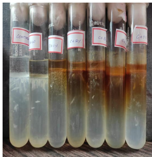
Fig 7: The inhibition effect of different concentrations of synthesized zinc oxide nanoparticles on struvite crystal formation was evaluated. Group (a) represents the control containing only magnesium acetate, showing no inhibition. Group (b) included water, and group (c) included ethanol, serving as solvent controls. Groups (d) through (h) correspond to increasing concentrations (1%, 2%, 3%, 4%, and 5%) of synthesized zinc oxide nanoparticles. A concentration-dependent inhibition of struvite crystals was observed, with the highest inhibition recorded at 5% nanoparticle concentration.
