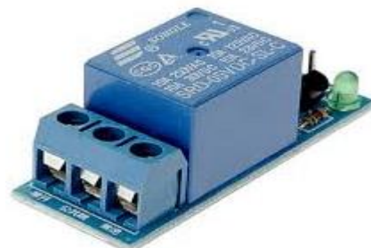
Fig. 7 Relay enabled on Board
