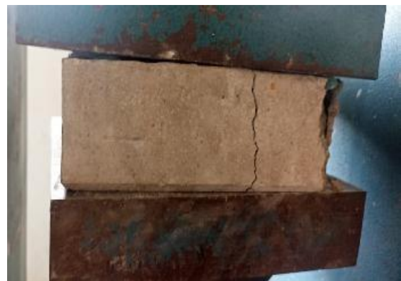
Fig 8 Testing of specimen (paver) in UTM
