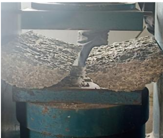
Fig 10 Testing of specimen (cylinder) in UTM
