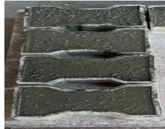
Fig 2 Casting of Blocks (260mmX160mmX60mm)
