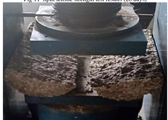
Fig 12 Testing of specimen (cylinder) in UTM
