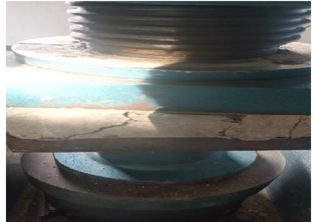
Fig 6 Testing of specimen (paver) in UTM
