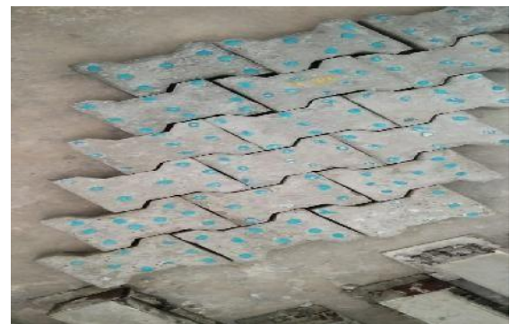
Fig 3 casted paver blocks
