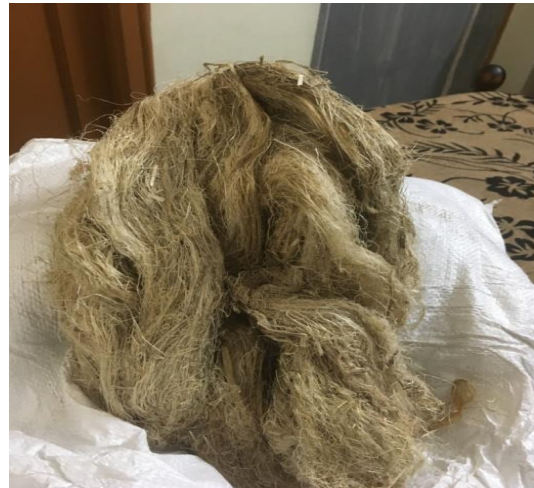
Extraction of pineapple leaf fibre
