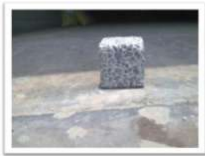
Figure 6 View of Specimen After Subjected to Chloride Attack
