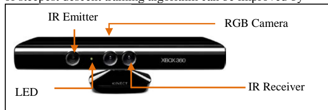
Fig. 1. Kinect sensor depicting camera and sensors.
