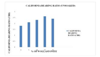
Figure 5: Comparison of various % of wollastonite and its california bearing ratio (CBR)
