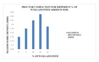
Figure 2: Comparison of various % of wollastonite and its maximum dry density (MDD)
