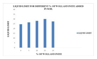
Figure 1: Comparison of various % of wollastonite and its liquid limit
