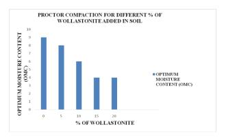
Figure 3: Comparison of various % of wollastonite and its optimum moisture content (OMC)
