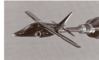
Fig 2 Balance with Model and support system
