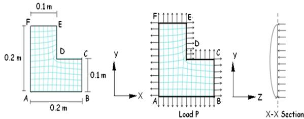
**Figure 1(b):** Geometry and pre-stress of L-shaped
