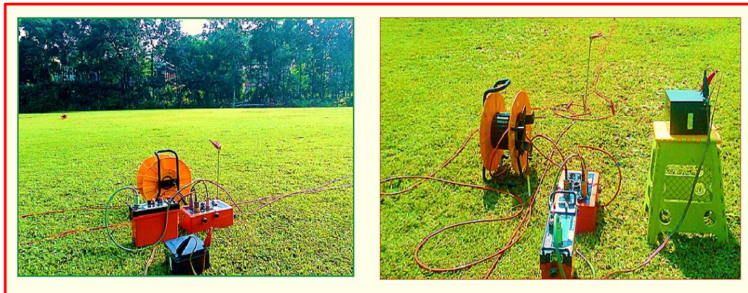
Figure- 13: shows the SAS1000 system, manufactured by ABEM Inc. of Swedish
