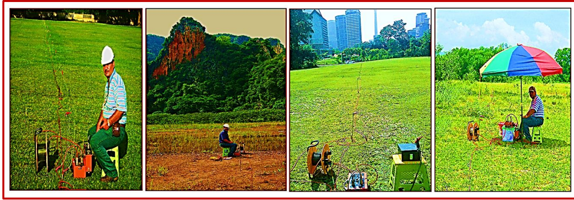
Figure 14: shows the typical setup for a 2-D survey with a number of electrodes along straight line attached to a multi-core cable in different sites in Kuala Lumpur and Selangor
