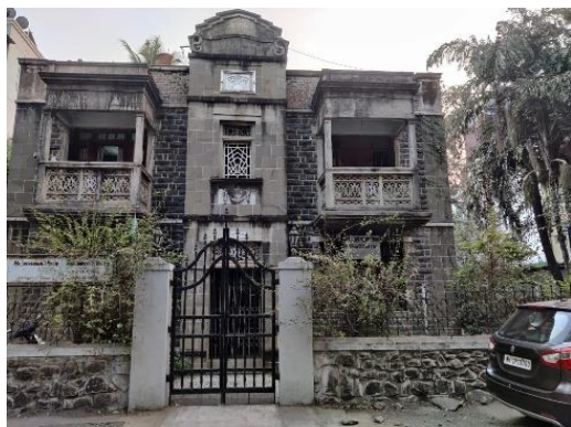
Fig. 4. This residential structure is a hybrid of many styles showing projecting balconies with stone railings. Central staircase stands out with art deco styled metal grills for staircase block and renaissance pediment, and combination of ashlar and rusticated stone masonry.
