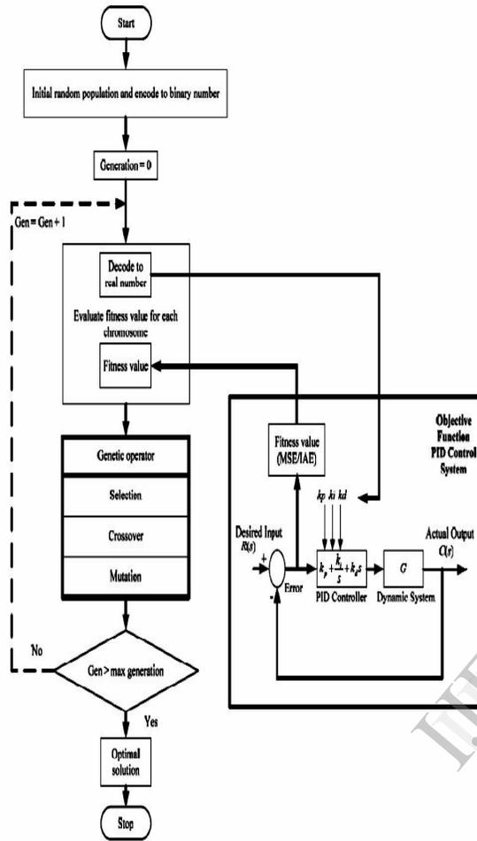
Fig.1. Genetic algorithm approach in tuning PID
