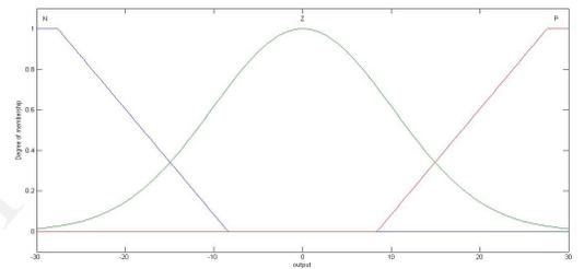
Fig.3. membership functions for input-change in error Variables
