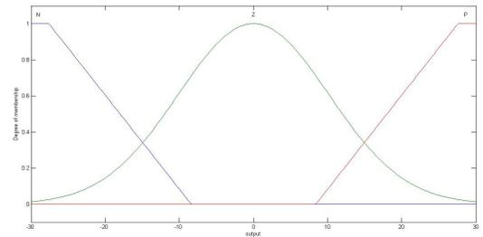
Fig. 4.Gaussian Membership Functions for Output Variable
