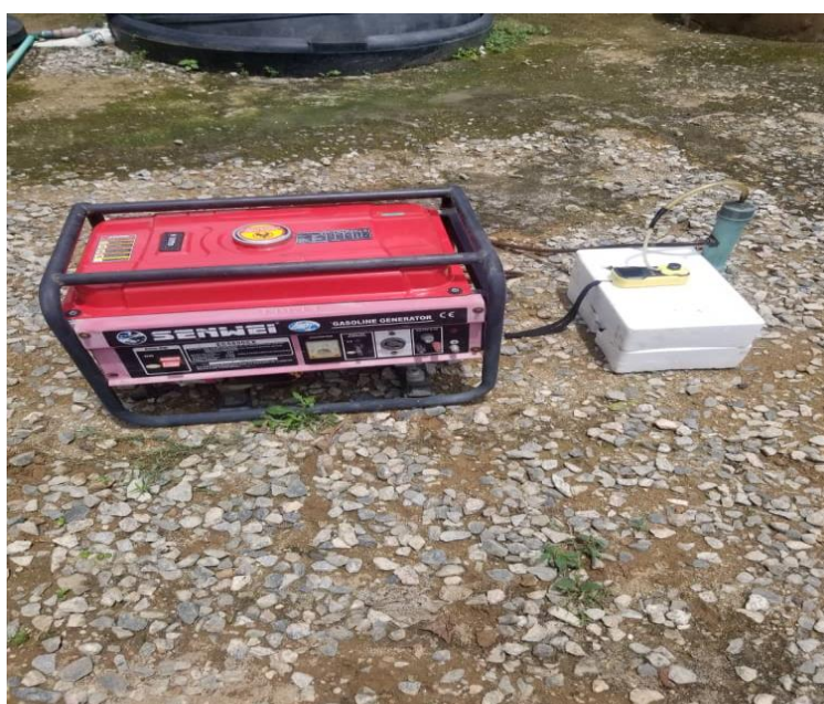
Plate 1: Experimental Setup for the Investigation of the activated carbon removal efficiency of the toxic gaseous emissions from gasoline-powered generator
