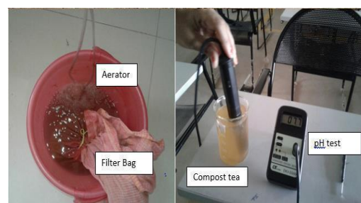
Figure 4 Aeration process setup & pH meter
