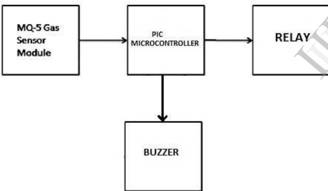
This block is placed near the houses to detect the gas leakage and cut off the AC power supply to the house on detecting a leakage. An alarm is also provided to alert the people.
