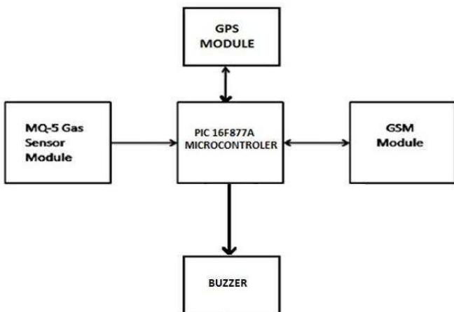
This block is placed on the body of gas tanker. The objective of this circuit is to send an alert message to emergency number on detection of a gas leakage. The message include warning for gas leakage and the location of lorry.
