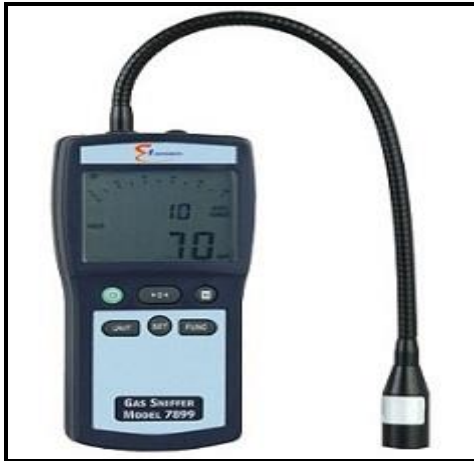
Figure(3)- Automatic fire damp detector
