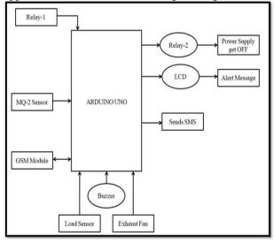
In the monitoring system, the LPG cylinder is considered where the application is using the load sensor to weigh the cylinder. If the threshold value which is set to 3Kg is greater than the volume of the Cylinder, then the signal is sent to Arduino Uno which then proceeds the signal to the GSM modem which will send the SMS to the agency for booking of the Gas cylinder. It is then stored the status of the booking the web page which will be easier to use.
